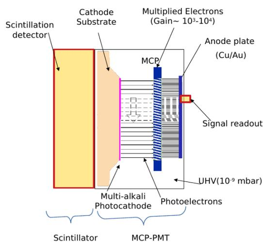
FIG. 1: Design of MCP-PMT depicted with different parts and its coupling to the scintillator.
