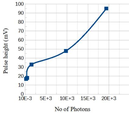
FIG. 3: The measured anode signal when the photons from a light source incident on the MCP-PMT.
