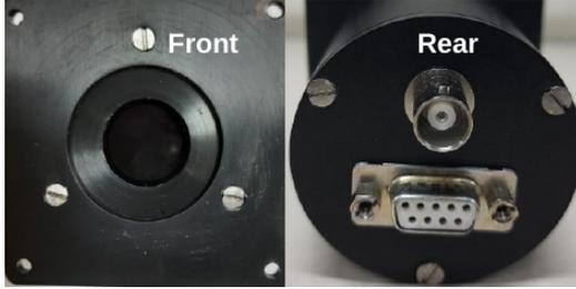
FIG. 2: The indigenously developed MCP-PMT showing front view (window of the PMT) and rear view (BNC connector for anode signal).
