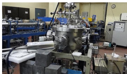
Fig. 1 External PIGE set up at FOTIA, BARC showing the HPGe detector and beam extraction window
