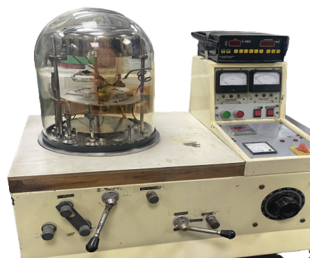
Fig. 1: Diffusion pump based coating unit used for the evaporation of ^{82}\text{Se} on ^{197}\text{Au} foil at the Department of Physics & Astrophysics, University of Delhi, New Delhi, India.
