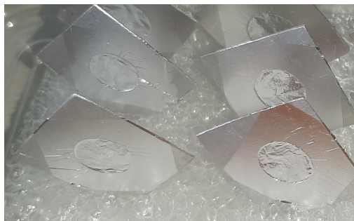
FIG. 2: Evaporated LiF on self supporting Ag foil
