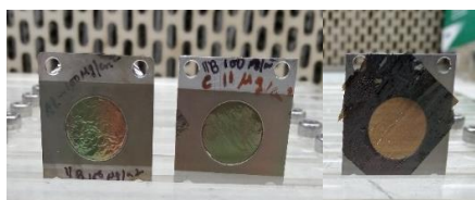
Fig. 2 ^{11}\text{B} targets on ^{27}\text{Al} backing (left), on ^{12}\text{C} backing (middle), self-supporting with natural B (right)
