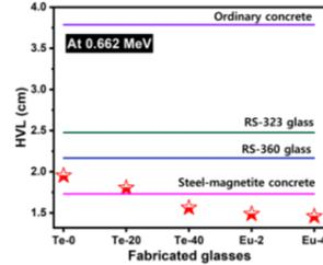
**Fig. 2.** HVL values compared with commercial radiation shields
