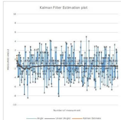
FIG. 4: Estimation of orientation of robot from IMU sensor data using Kalman Filter
