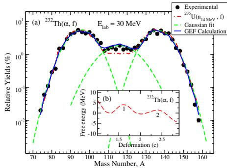
FIG. 2: (a) Even-Z,N mass yield distribution profile obtained from the reaction,  $^{232}\text{Th}(\alpha, f)$ . (b) Calculated free energy profile as a function of deformation parameter of the system. Details have been discussed in Ref.[2].
