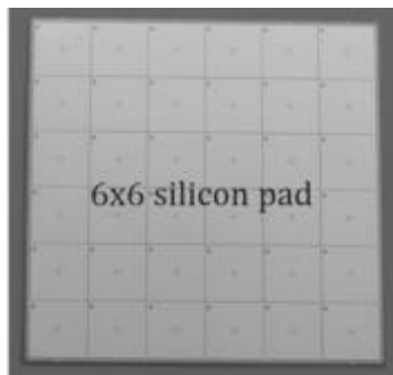
Fig 1: Diced 6x6 silicon pad (individual element of 1 cm 2 )
