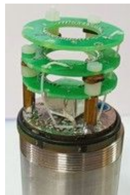
Fig.2: Assembled Gas-CsI detector
