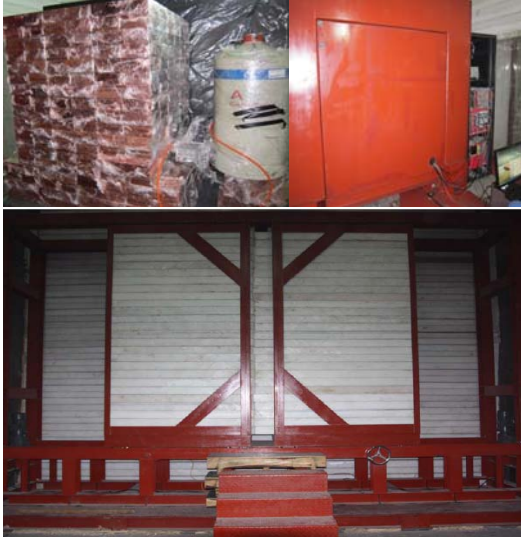
Fig. 3: The 4x5g ULE-ULB-HPGe detector enclosed by copper, lead and boron loaded polyethylene shielding respectively in clockwise direction from top.
