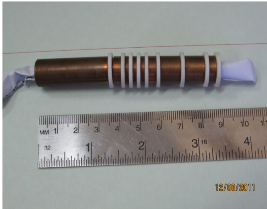
Fig 2: Electrode assembly of trapping zone with MACOR spacers machined at VECC.
