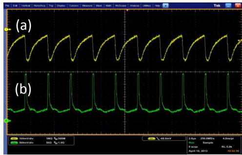
Fig. 5 tail pulse input to preamplifier and Shaper output at 500Khz and Vbfb=6, Input charge = 50fc
