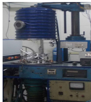
FIG. 1: The diffusion pump based coating unit
