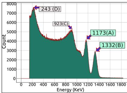
FIG. 2: a)  $^{60}\text{Cobalt}$  gamma spectrum calibrated using the known photopeaks labelled A & B . The compton edge corresponding to 1173keV photopeak and backscatter peak calculated with this calibration are also labelled as C & D respectively.
