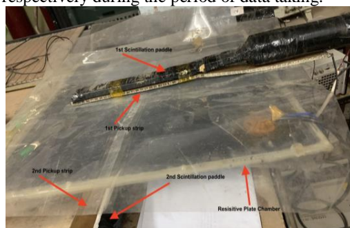
Fig.2: Experimental setup of RPC detector for efficiency measurement.
