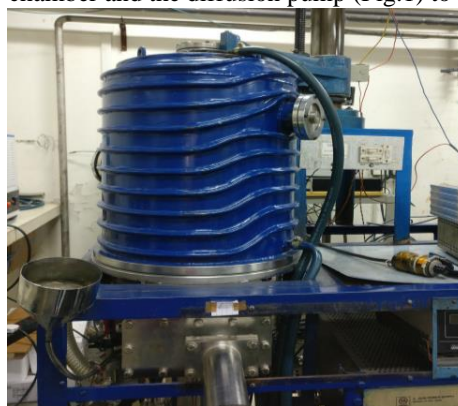
Fig. 1 Chamber used for fabrication of Nat,64 Zn targets
