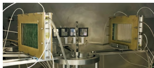
FIG. 5: Setup for fission gated light charged particle experiment.
