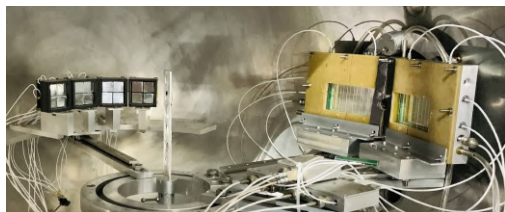
FIG. 3: Schematic of CsI and MWPC setup at NAND.
