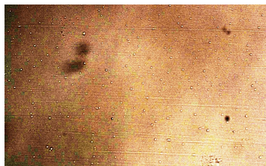
Figure 1: Figure show particular image of alpha tracks for 5.48 mev alphas
