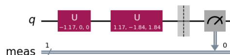
FIG. 1: Quantum circuit for simulating two-flavor neutrino oscillations using the virtual- Z gate. We perform the simulation in both Qiskit Aer simulator and IBM Q machine.
