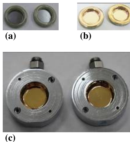
Fig.1: (a) After preparing and mounting samples (b) Samples after metallization (c) Detectors after encapsulation
