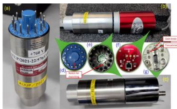
FIG. 1: (a) Typical CeBr 3 detector with PMT, (b) CeBr 3 detector with Osprey, (c) CeBr 3 detector with 2007P, (d) PIN side of PMT, (e) socket side of 2007P and Osprey tube base, (f & g) connection side of Osprey and 2007P, respectively.
