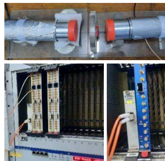
FIG. 1: (Top Panel) Setup of two B380 LaBr 3 (Ce) detectors at the UGC-DAE CSR, Kolkata Centre. (Bottom Panel, Left) 12-bit 250 MHz PIXIE-16 digitizer modules. (Bottom Panel, Right) 12-bit 500 MHz digitizer module that has recently been added to the setup.
