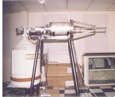
Fig. 2: The mating of the Si(Li) detector with Vacuum chamber
